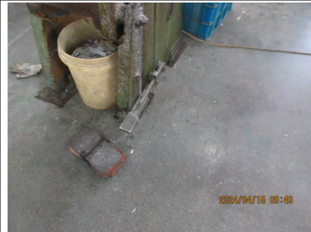
NC7.17 40% punching machines' pedals missed protective covers
