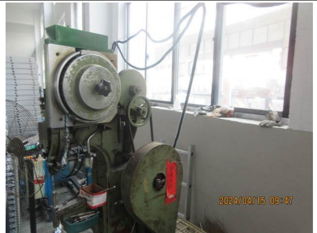
NC7.17 All riveting machines' pulley protection covers were incomplete
